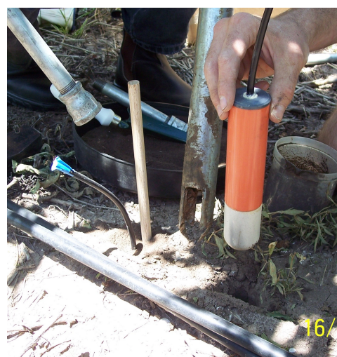
Figure 2. Field installation of the extractor in a vineyard
