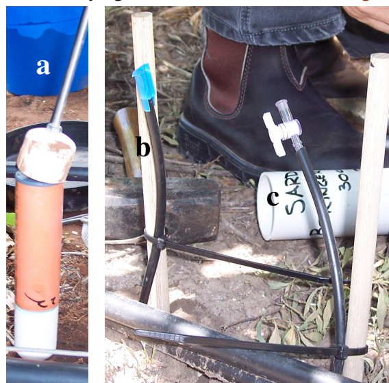
Figure 4. (a) Insertion tool (b) wooden pegs and (c) PVC encasing
